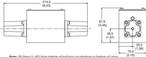
Note: 30.0mm (1.18") from bottom of bolt hole counterbore to bottom of valve.
