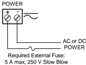
**Figure 4: Power Connections**
