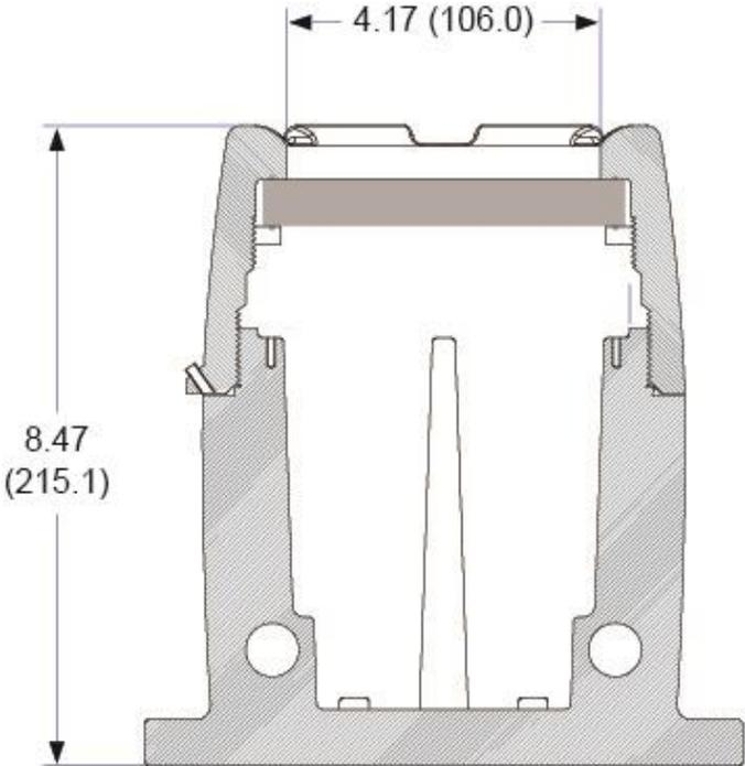
Figure 22: Enclosure Dimensions – Side Cross Section View
