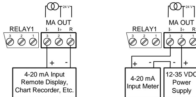
Figure 16: 4-20 mA Output Connections
