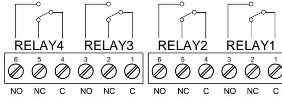
Figure 12: Relay Connections
