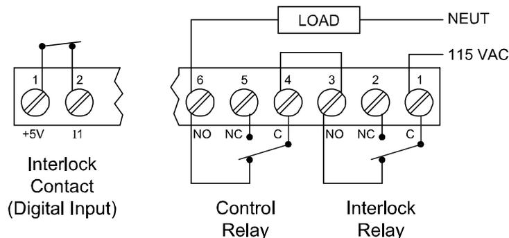
Figure 17: Interlock Connection
