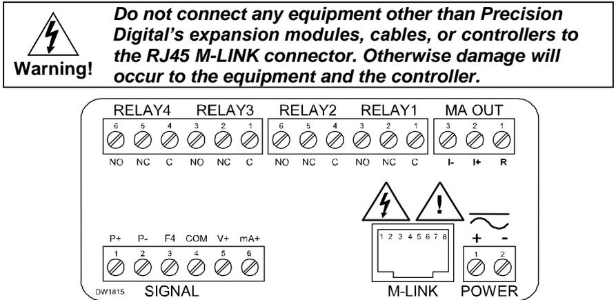
**Figure 3: Connector Labeling for Fully Loaded PD8-6210**
