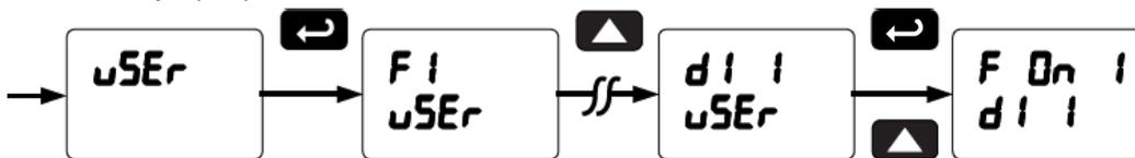
3. Connect a switch or dry contact between the +5V terminal and the corresponding digital input (d1-1 to d1-4) terminal.
