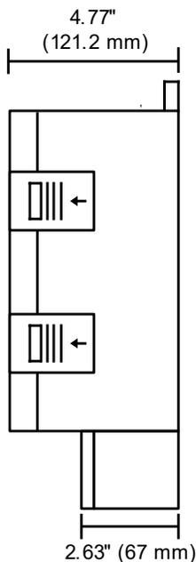
Figure 2. Meter Dimensions - Side View
