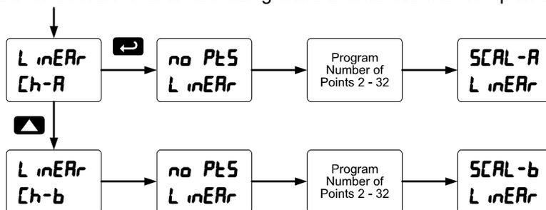
Note: After Scale is displayed continue pressing the Enter button until the meter completes the scaling of the input and display values.
