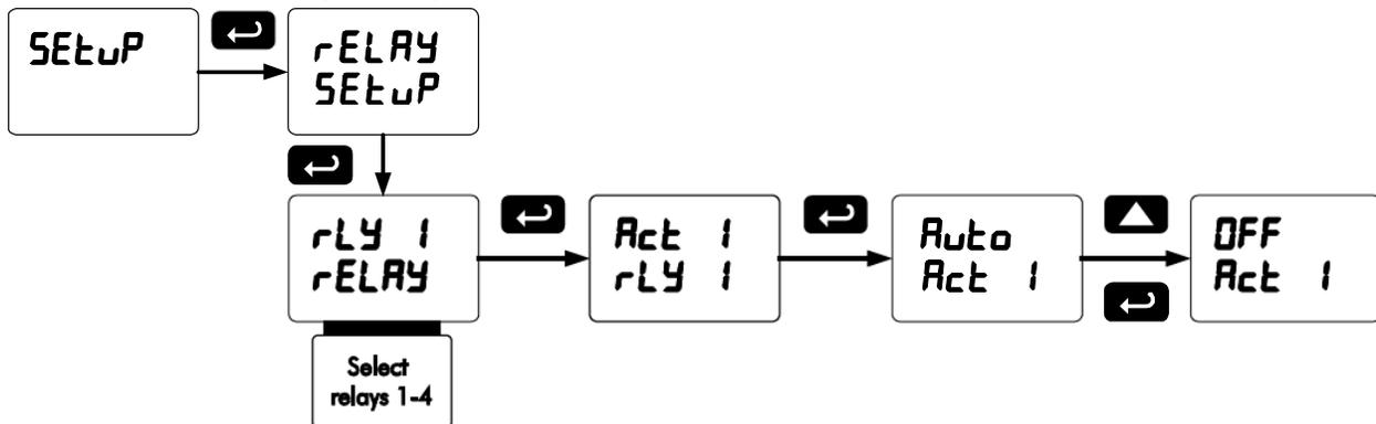
2. In the *Advanced features – User* menu program any of the digital inputs to *Force On* any of the internal relays (1-4).
