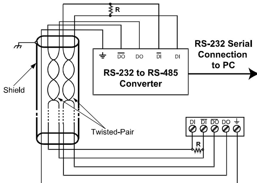
Figure 15. RS-422 or RS-485 Wiring
