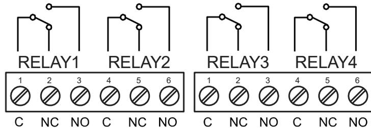
Figure 12. Relay Connections
