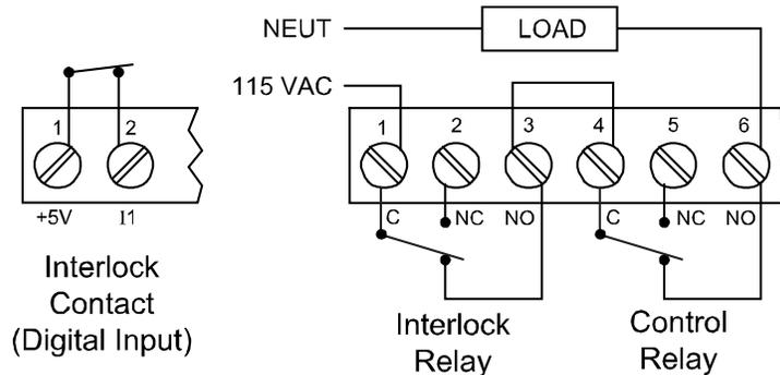
**Figure 22. Interlock Connections**
