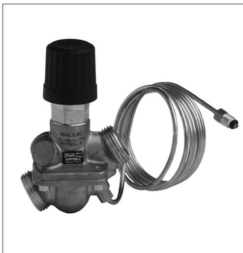
The controller has a control valve with adjustable flow restrictor, connection neck for electrical actuator, and an actuator with one control diaphragm.
