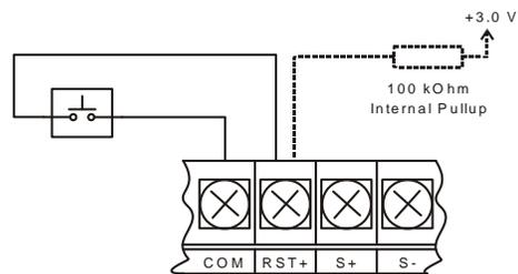
Figure 9. Reset Connections
