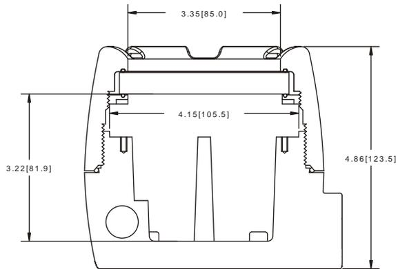
Figure 17. Enclosure Dimensions – Side View
