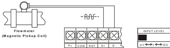
Figure 4. Self-Powered Magnetic Pickup Coil Flowmeter (Coil)
