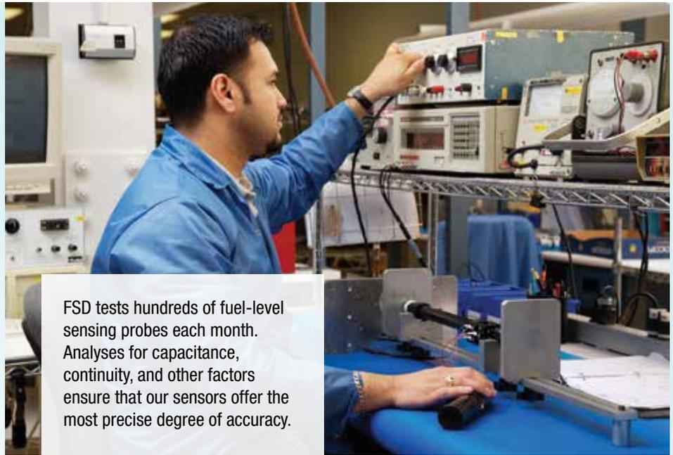
FSD tests hundreds of fuel-level sensing probes each month. Analyses for capacitance, continuity, and other factors ensure that our sensors offer the most precise degree of accuracy.
