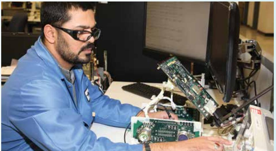
*Circuitry for FSD's fuel quantity gauging and management computers is thoroughly tested on in-house-developed equipment to verify correct input and output readings. Our components are tested to exceed all OEM specifications.*
