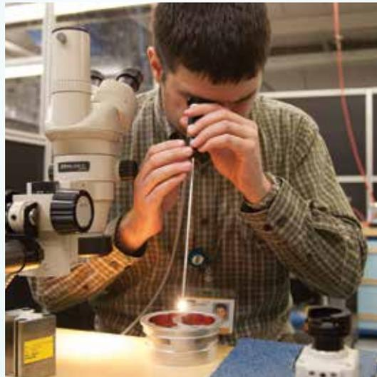
Visual inspections of pump components are crucial after qualification testing to determine if damage or wear is present.
