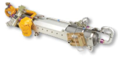
Single-aisle air separation module pallet
