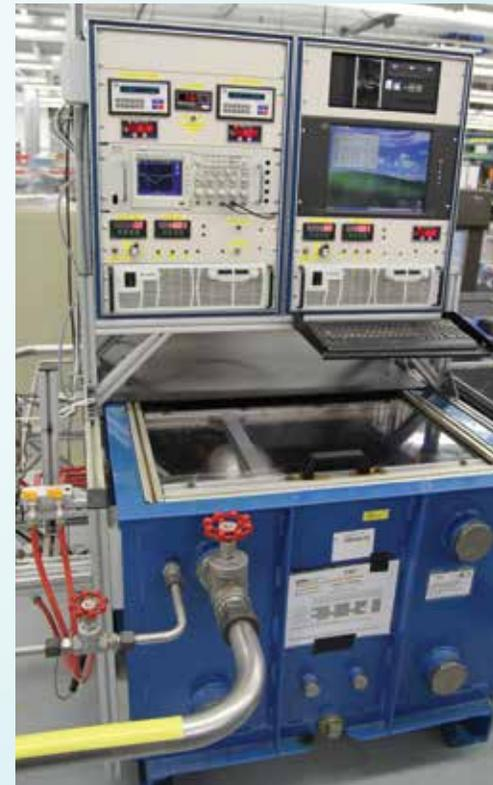
Production test tanks throughout FSD are used to evaluate pumps to document performance characteristics.
