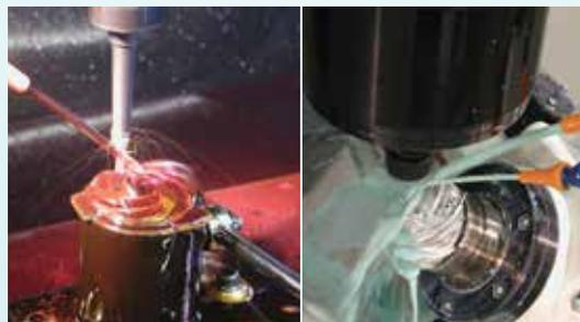
FSD's multi-use model shop routinely machines parts, including pump impellers, using various cutting tools, oil, and coolants.
