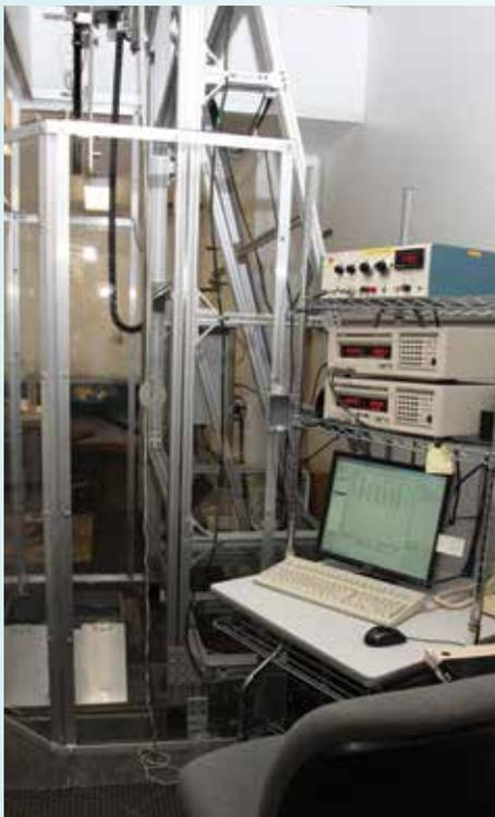
*FSD's test stands for in-tank gauging components allow us to simulate a fuel tank environment. Calibration fluid is used to avoid the inherent combustion risks of using fuel.*
