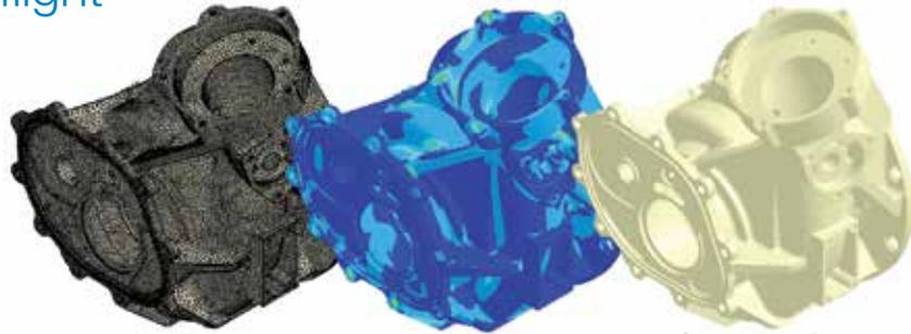
1) The finite element analysis (FEA) mesh rendering allows the isolation of minuscule elements to calculate stresses in complex geometries.
