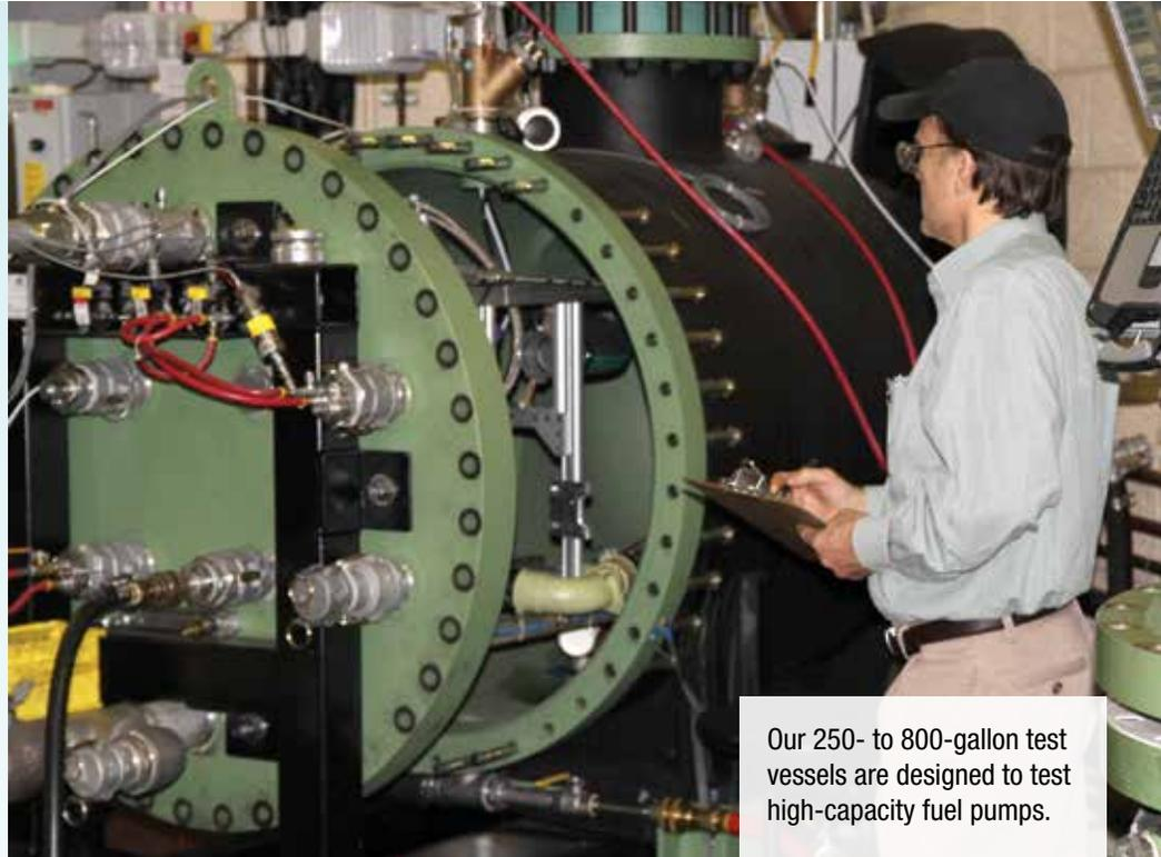
Our 250- to 800-gallon test vessels are designed to test high-capacity fuel pumps.
