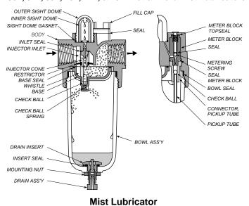
**OUTER SIGHT DOME** FILL CAP INNER SIGHT DOME METER BLOCK SIGHT DOME GASKE BODY METER BLOCK INLET SEAL SEAL INJECTOR INLE METERING INJECTOR CONE RESTRICTOR SEAL BASE SEAL METER BLOCK BOWL SEAL BASE CHECK BALL CONNECTOR, PICKUP TUBE PICKUP TUBE BOWL ASS'Y DRAIN INSERT INSERT SEAL MOUNTING NUT
