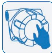
The ProtEX-MAX is equipped with four sensors that operate as through-glass buttons so that it can be programmed and operated without removing the cover (and exposing the electronics) in a hazardous area. The SafeTouch buttons are configured by default to duplicate the function of the front panel mechanical pushbuttons associated with the integrated meter.
